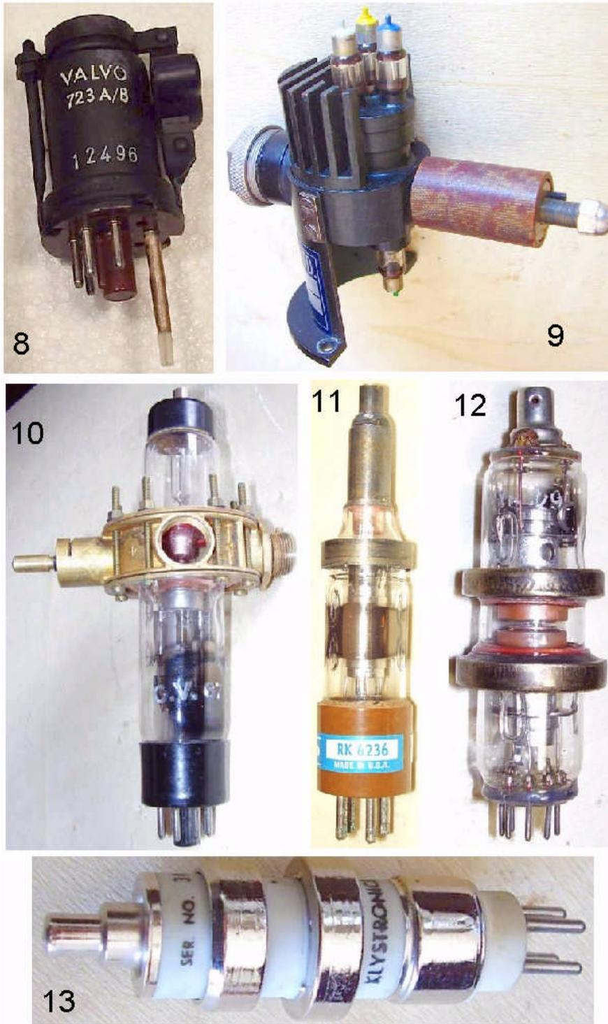
**Table II - Pic. 8:** 723A/B was the predecessor of 2K25. **Pic. 9:** 8RK8 from Elliot-Litton, GB, is a K-band reflex klystron. **Pic. 10:** CV67 was one of the typical WWII British klystrons, with the factory assembled external cavity. **Pic. 11:** 6236 tunes from 3.8 to 7.6GHz. **Pic. 12:** EMI VX5089 tunes from 1.8 to 4.5GHz with external cavity. **Pic. 13:** ZV1009 'Velocitron' from Polarad is a ruggedized version of the 6BL6, tunable from 1.5 to 6GHz.
