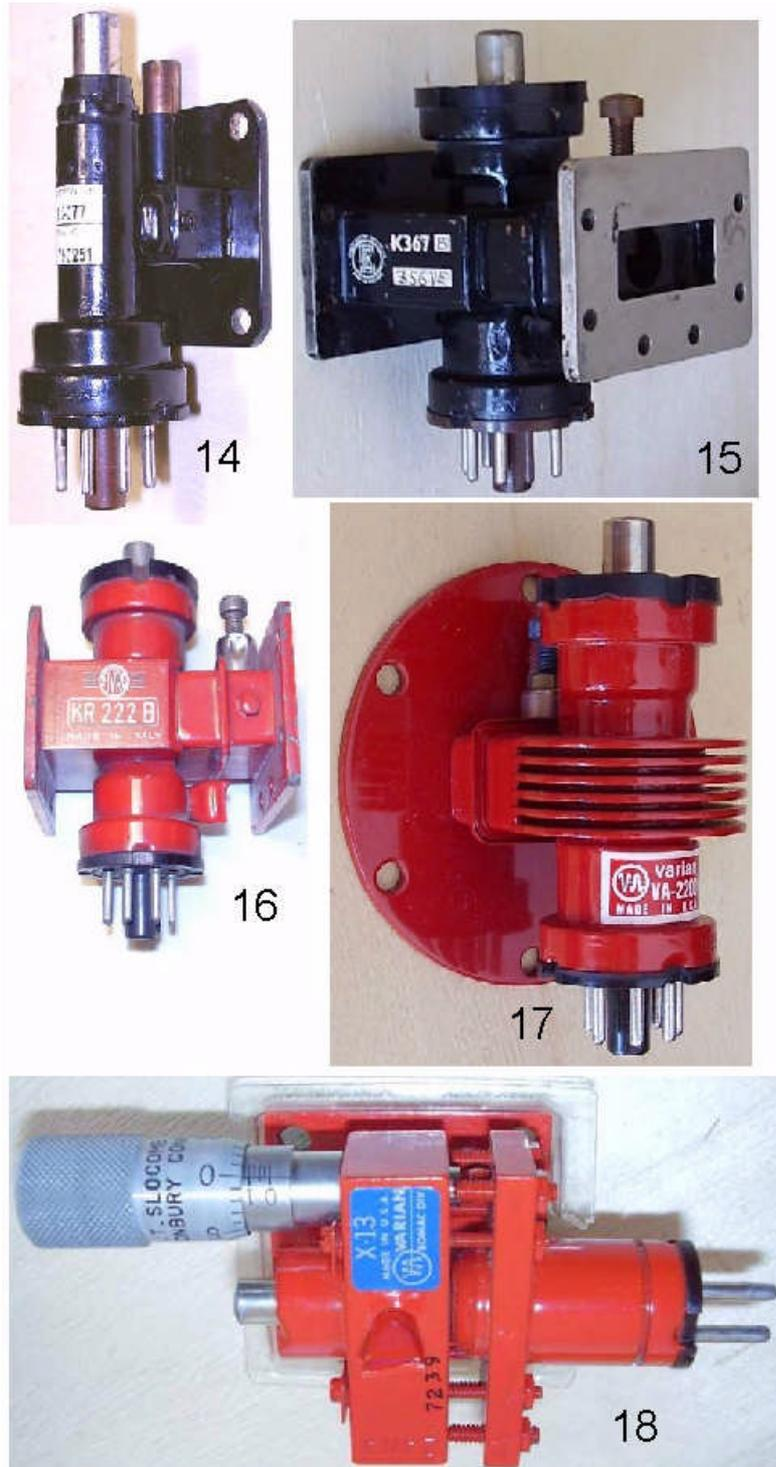
**Table III – Pic. 14:** EEV K3077 X-band oscillator for doppler use. **Pic. 15:** EEV K367B is a reflex oscillator used in communication relay links. **Pic. 16:** Fivre KR222B is another klystron for microwave relay; 1W at 7125 to 7425MHz. **Pic. 17:** Varian VA220D, a further klystron for microwave relay systems. **Pic. 18:** Varian X-13 is a precision X-band oscillator, with micrometric tuning.
